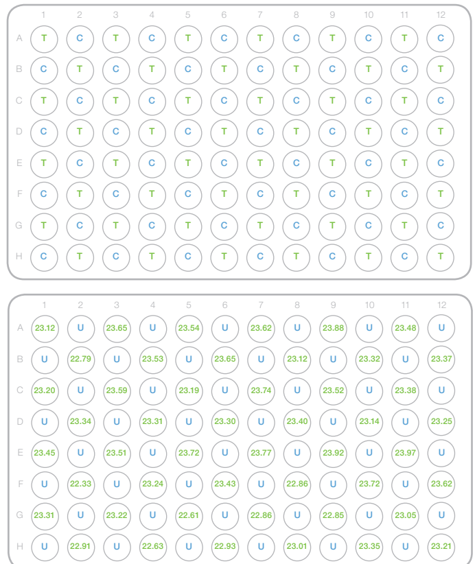
Figure 2: (top) samples with different DNA concentrations were set up in a checkerboard pattern (control, template) on the 96 well plate and subjected to temperature cycling; (bottom) after cycling, no cross-contamination could be detected by qPCR in the control wells (U).
